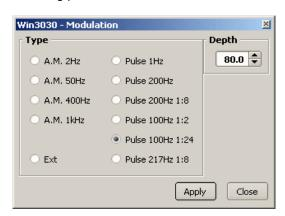
For the AM types it is also possible to adjust the depth of modulation.
