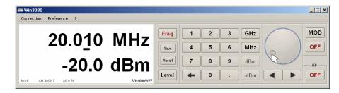
The value over the cursor can be changed by pointing and rotating the graphical knob on the screen with the mouse or using the arrow keys on the keyboard of your PC.
