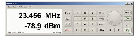
Press RF button to switch the output ON or OFF.
