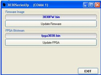
During the storing procedure, a blue bar will progress from left to right in the window of the PC, showing percentage of downloading time by time until 100%.
