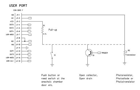
Fig. 2-2 Example of INTERLOCK circuits
