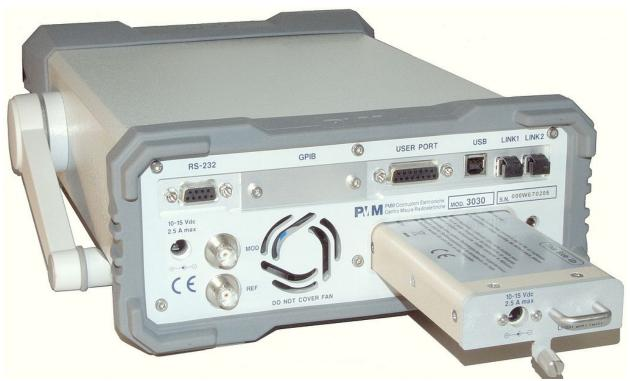
Fig. 1-5 BP-01 Replaceable Battery
