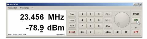
Press the button under MOD to switch ON or OFF the modulation selected.
