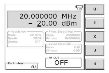
The frequency step of the rotary knob can be directly edited into this window, inputting data through the five Function Keys as usual.
