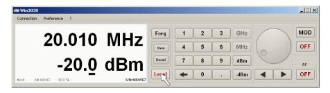
The frequency and level values can also be entered using the softkeyboard. After entering the digits, with the eventual decimal point, of the frequency value, it is necessary to press the unit among MHz and GHz.
