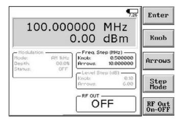
RF Out On-OFF The fifth button in the Frequency menu is used to switch the RF Output On or OFF.
